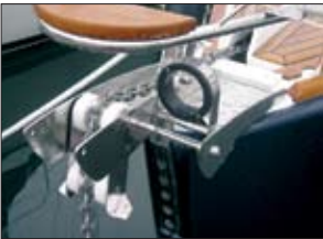
Bow bracket integrated with bow anchor fitting.
